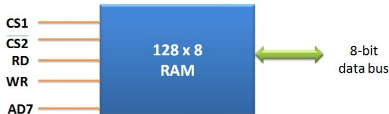
Block Diagram Representing 128 x 8 RAM (Random Access Memory)
